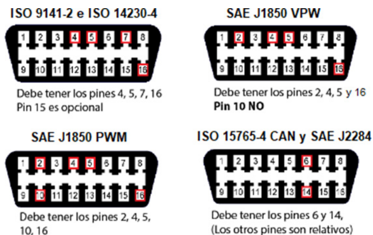
Figure 9. Connectors for OBDII protocols (23)
