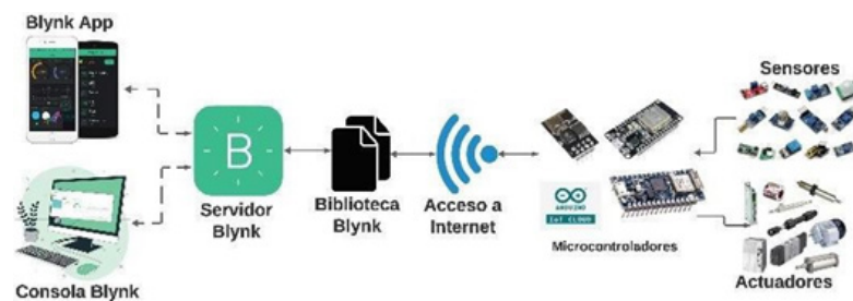
Figure 7. Integration of the Blynk platform with external devices
