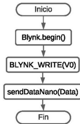
Figure 11. Flowchart for monitoring changes in virtual variables
