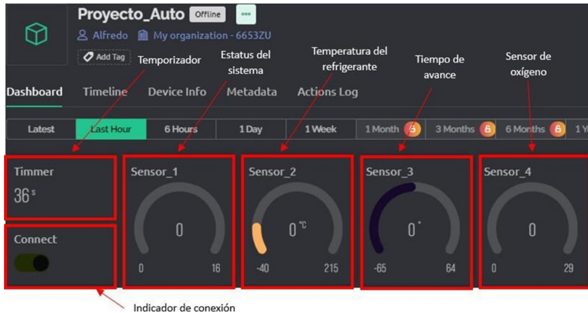
Figure 14. Display panel for the selected variables on the Blynk platform
