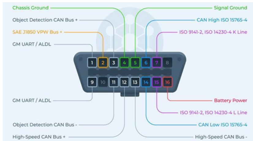
Figure 2. OBDII port pin designation with one or two CAN buses (9)
